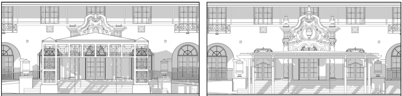
Figure 3: Existing (left) and proposed (right) elevation drawings of the porte cochere and restored portal.
